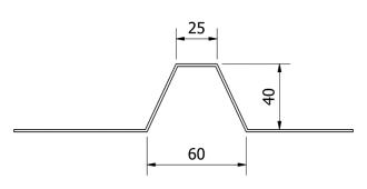
Steel sheet minimum thickness: 0.5mm
