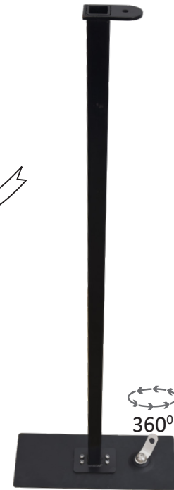
REF. FA 20 701 01 LG. 1.5 m MAT. STEEL Kg 10.45 KG Sys. KS 8000 / KS 9000
